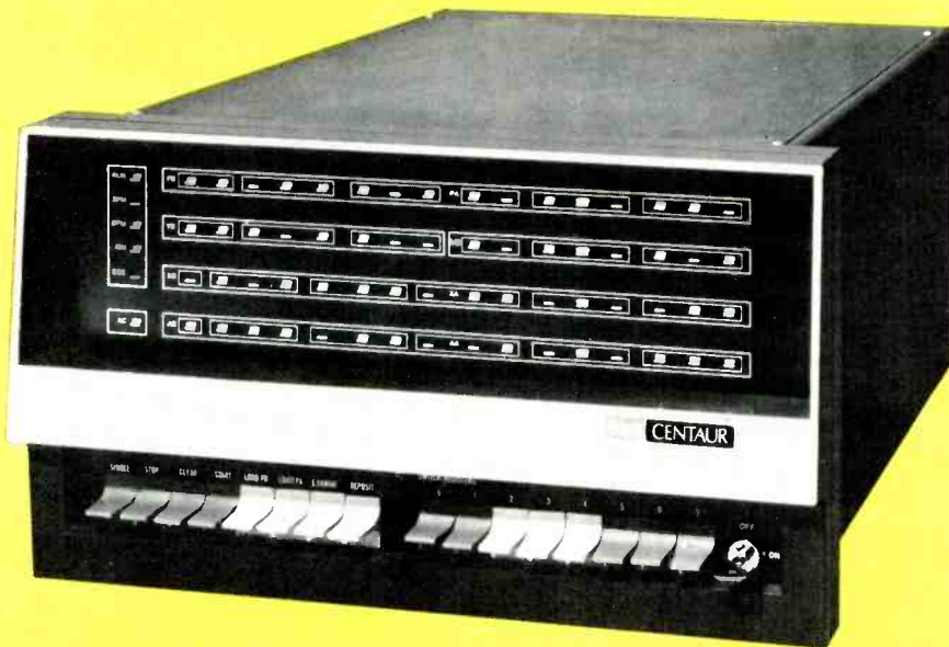
Fig. 1 The Foto-Mem Centaur mini-computer . . . at the heart of the WTIC election system.
