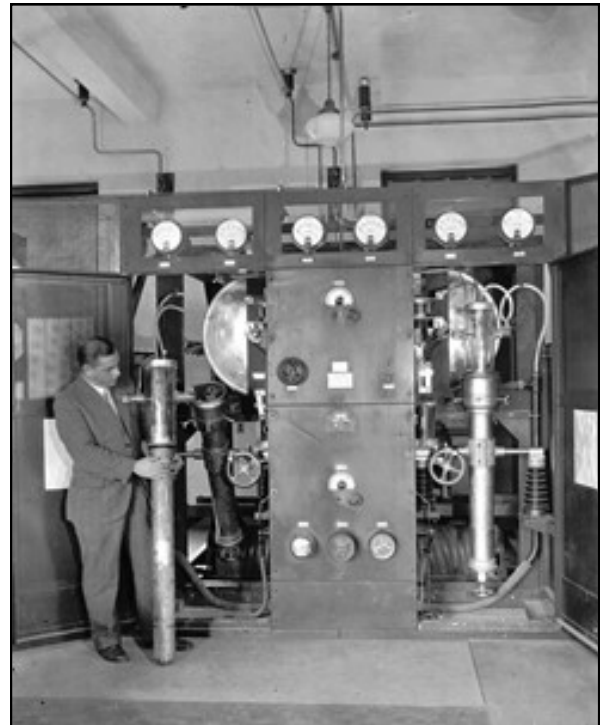
Most likely this is WTIC engineer H. M. O'Neill holding one of the huge water-cooled transmitting tubes. (From the WTIC promotional booklet.)
